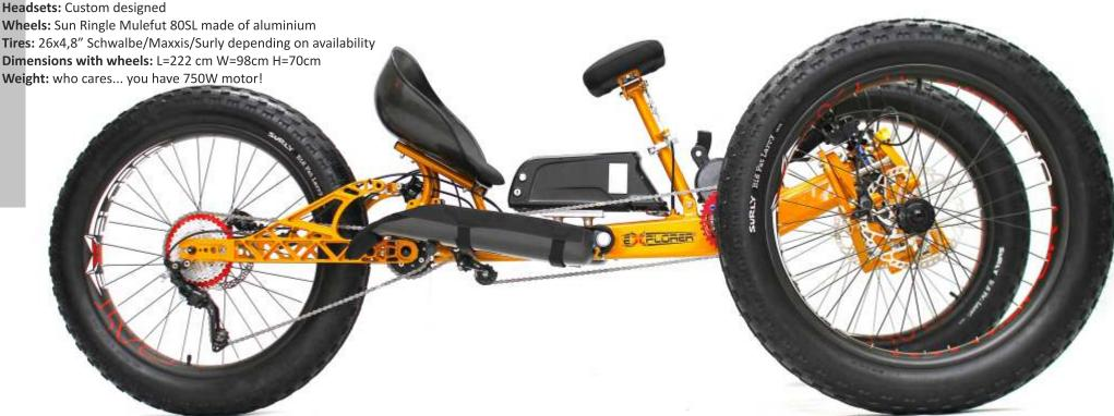
SPORT-ON proudly presents a FAT EXPLORER. This extraordinary handcycle is a upgraded version of our flagship off-road handcycle and is offered as a separate model, due the fact of many changes in design. FAT EXPLORER is factory equipped in a FAT WHEELS, 750W electric assist, CNC machined front and rear suspension and internal cable routing. This handcycle is unstoppable off-road, especially on soft surfaces like sand, mud or snow.
