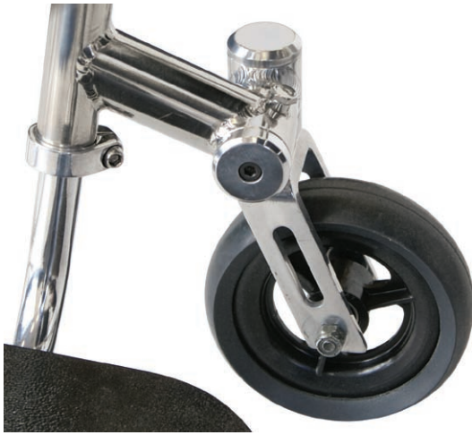
A castor with adjustable positioning is necessary when adjusting the squeeze and rake
